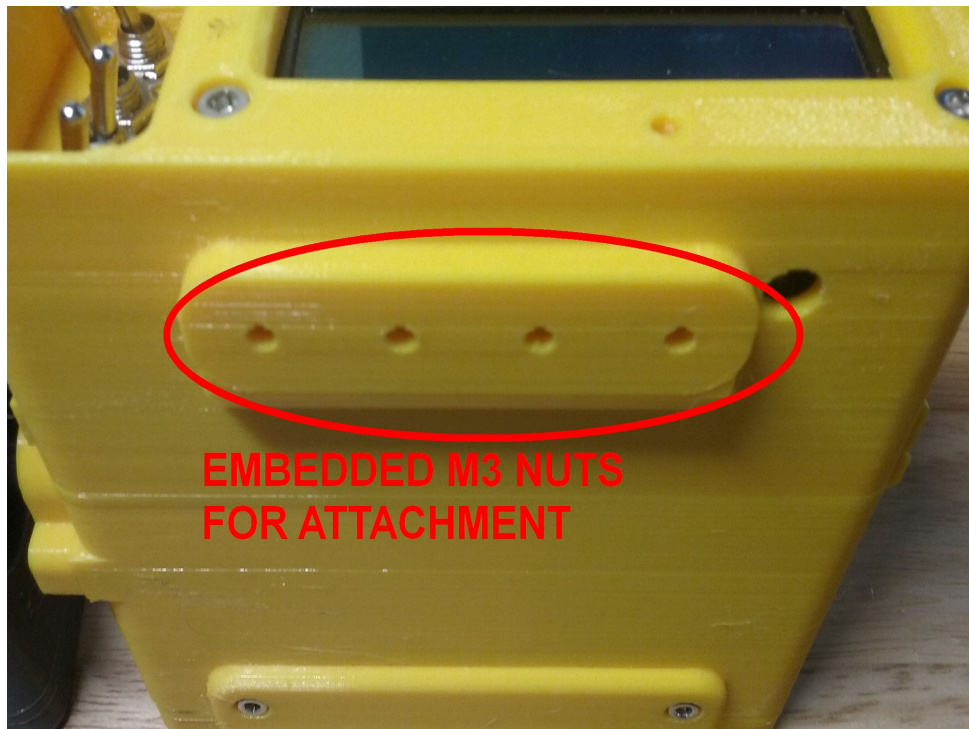
Illustration 6: Attachment points for belt loop, MOLLE panel, etc. Please note case is 3D printed, and is NOT waterproof
