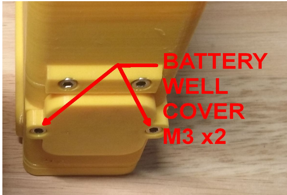
Illustration 5: Battery well cover. Please use care with fasteners; case is 3D printed
