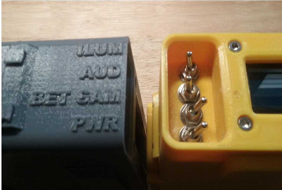
Illustration 2: Switch locations and functions. Labels are on LEFT side of case
