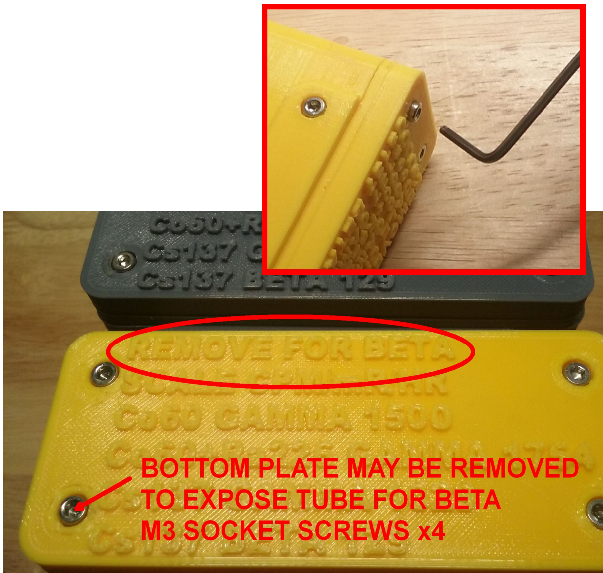
Illustration 3: Beta Window: Expose the tube inside, to measure beta radiation
