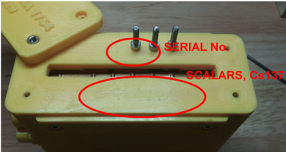
Illustration 1: Beta Window swung aside, showing tube, s/n, and scalar locations. Cap screws are size M3.
